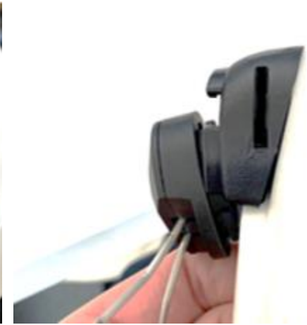
4. From the rear, the ear defender has fully worked itself out of position by rotating the ear defender more.
