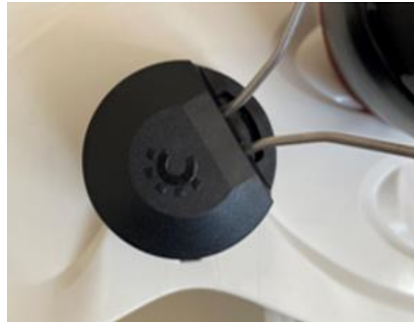
7. On rotation, the ear defender clip does not disengage or work its way out of the helmet mounted euro clip.
