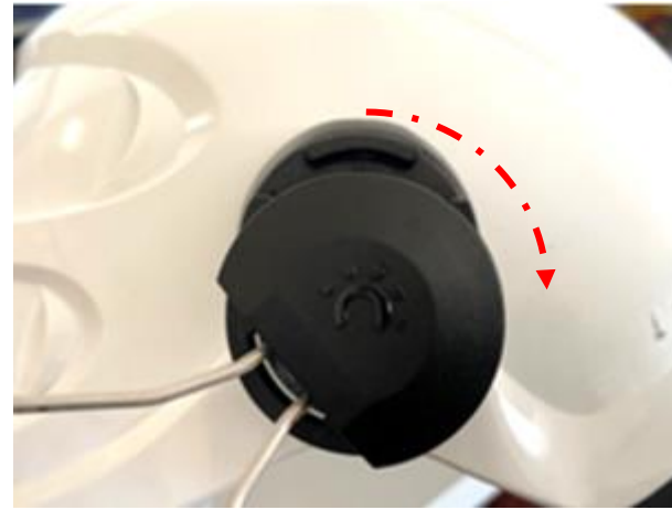
3. However, turning the ear defender, the clip works its way out of the helmet mounted euro clip.
