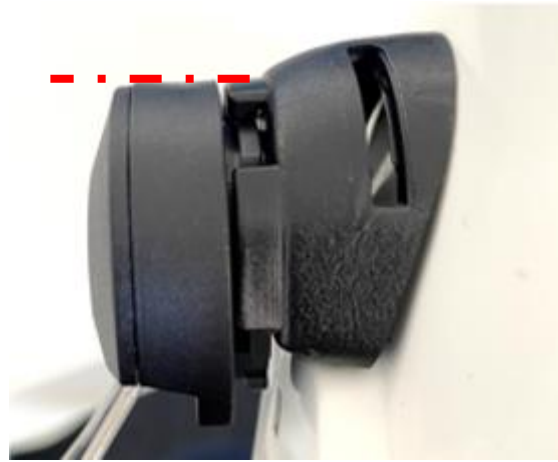
2. From the side, it also looks engaged. Clip top is flush (red dashed line) to the top of the helmet mounted euro clip
