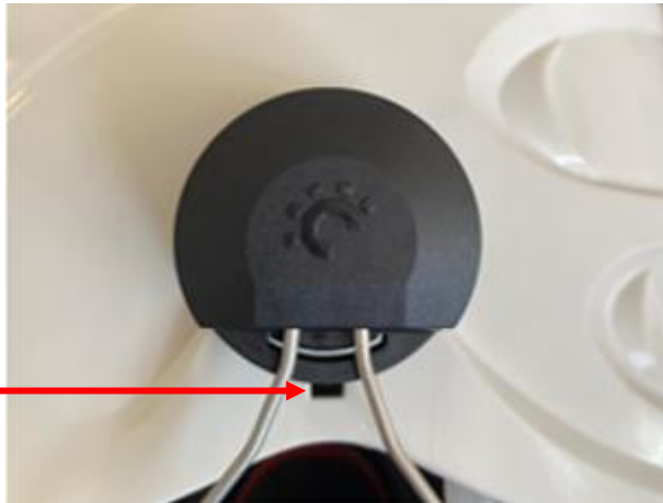
5. Engaging the ear defender clip – this position is engaged – the ear defender clip completely hides the helmet mounted clip. You can see more of the square slot on the helmet (indicated)
