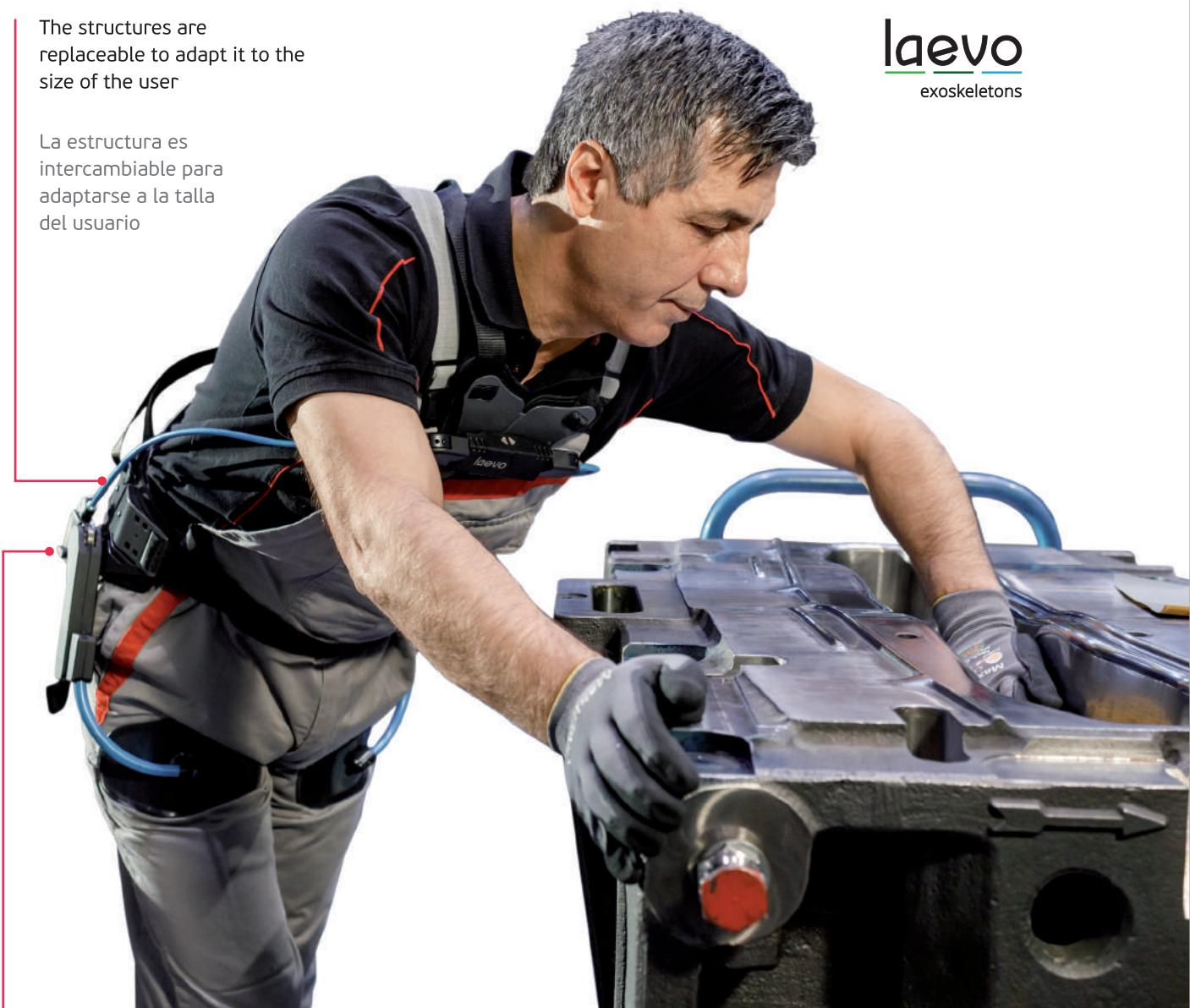
ON / OFF button that allows you to unlock the device to sit, drive forklifts, climb stairs
